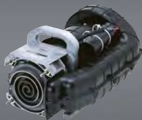
scroll air end (1HP) dryer (direct drive)
